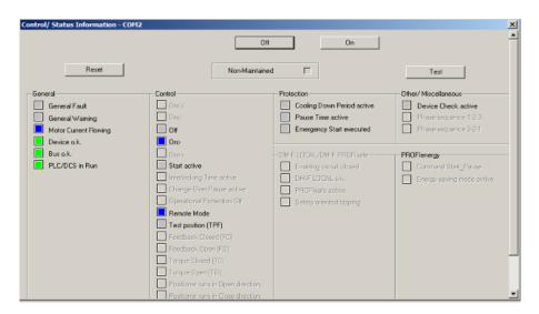
Figure 2.19. Interface for sensor initialization and motor check before starting [43]
