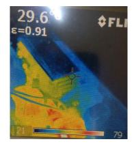
Figure 4.25. Overheating radiator with reduced fan speeds [78]
