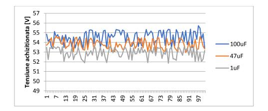
Figure 4.22.Acquisition of signals for different capacitor values (ZOOM) (gray -  $1\mu$ , red -  $47\mu$ blue -  $100\mu$ )
