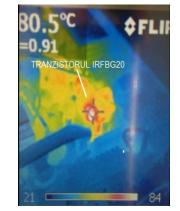
Figure 4.26. Temperature value of transistor with reduced cooling fan speeds [78]
