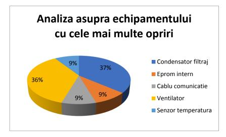
Figure 3.2. Analysis on the equipment with the most stops [49]
