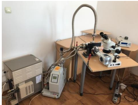
Figure 2.1: Measurement system used in the lab for the temperature sensors
